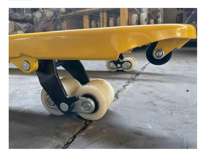
4. The steer and load wheels are engineered with high quality components and bearings to provide a low rolling resistance. The steer wheels rotate through a 200 degree range for easy maneuvering in tight spaces. Available as standard Polyurethane or optional Nylon to meet application needs.
